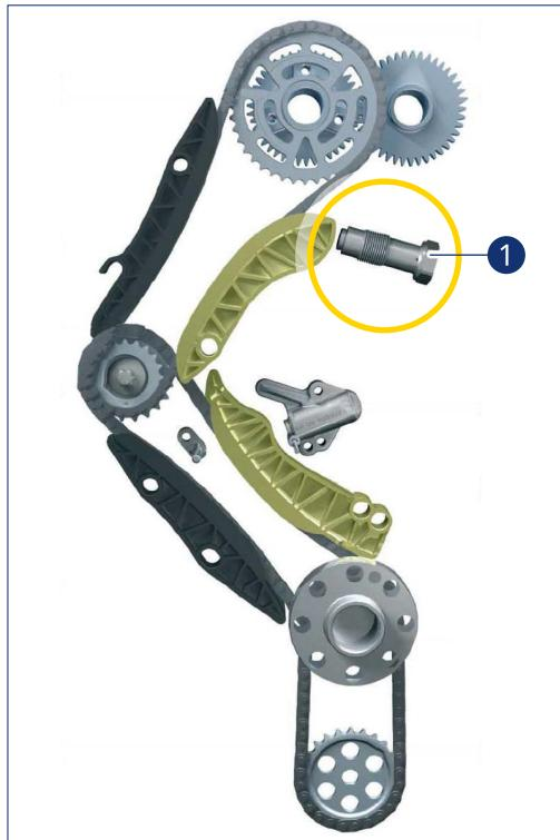
**On a limited number of vehicles**, this variation in length of the threaded shaft will require the housing on the head to be modified. This modification will be necessary in order to be able to correctly fit the tensioner.
